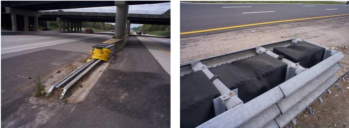
**Figure 3.16 – Impact Attenuators**
