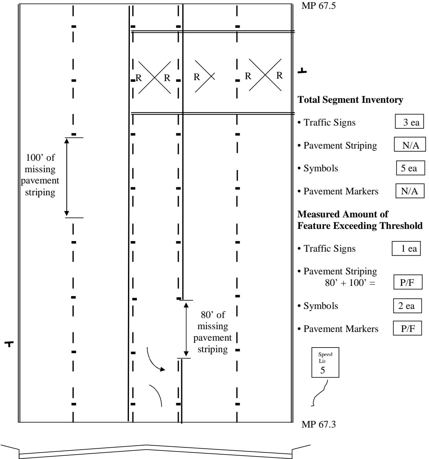
**Figure 3.26 – Example Roadway Conditions for Element 4**
