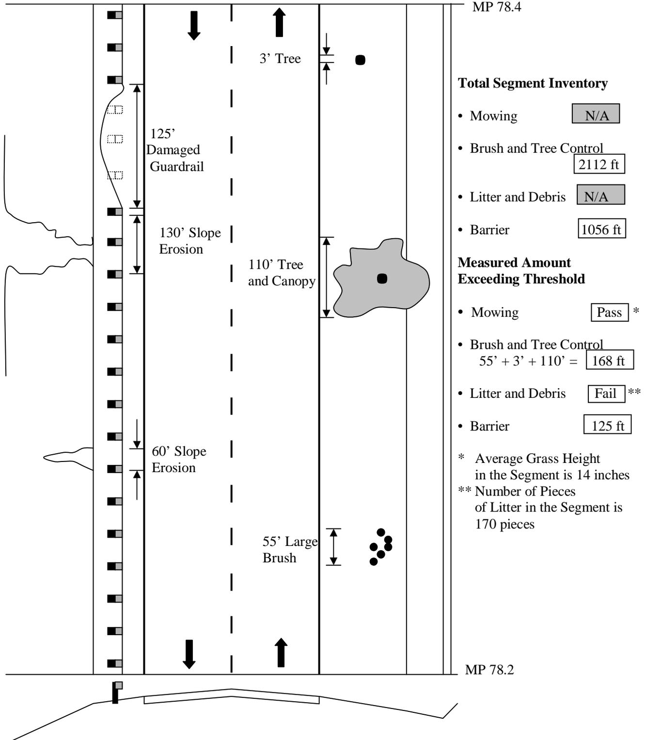
**Figure 3.19 – Example Roadway Conditions for Element 3**
