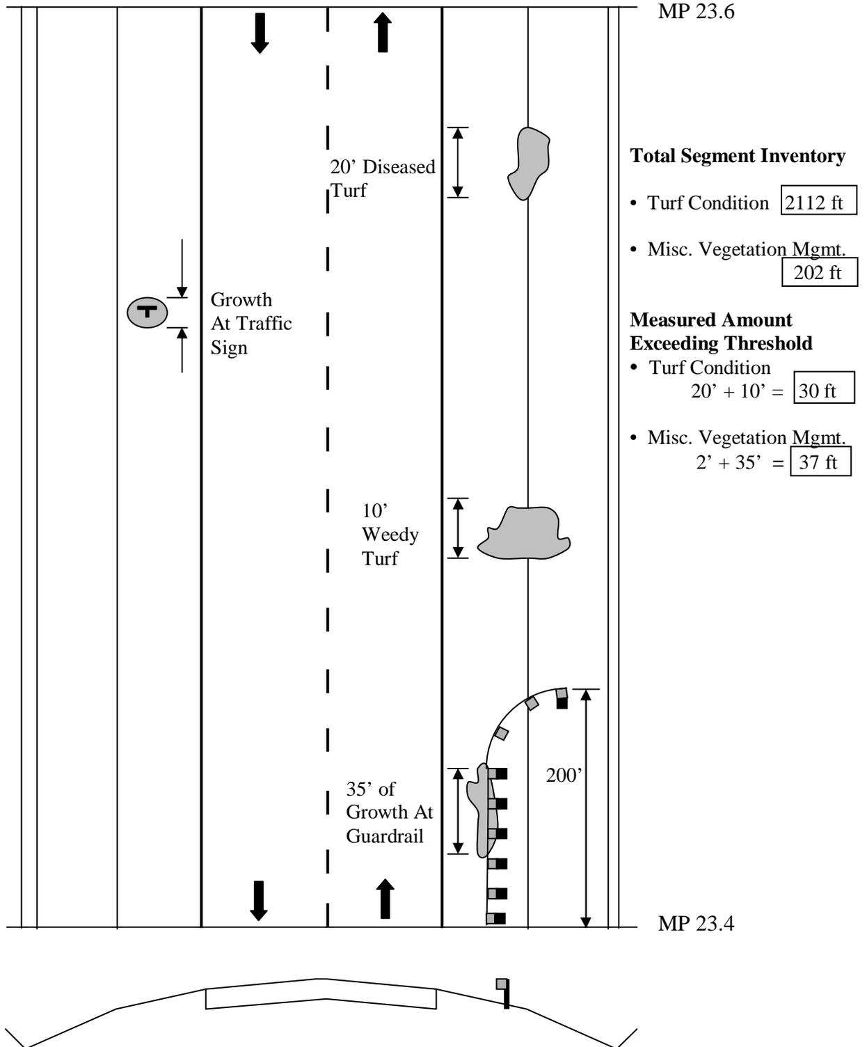
**Figure 3.29 – Example Roadway Conditions for Element 5**
